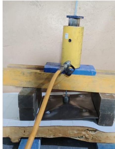
Figure 2b. Picture of NovaFlat specimen failure mode (System 1)
