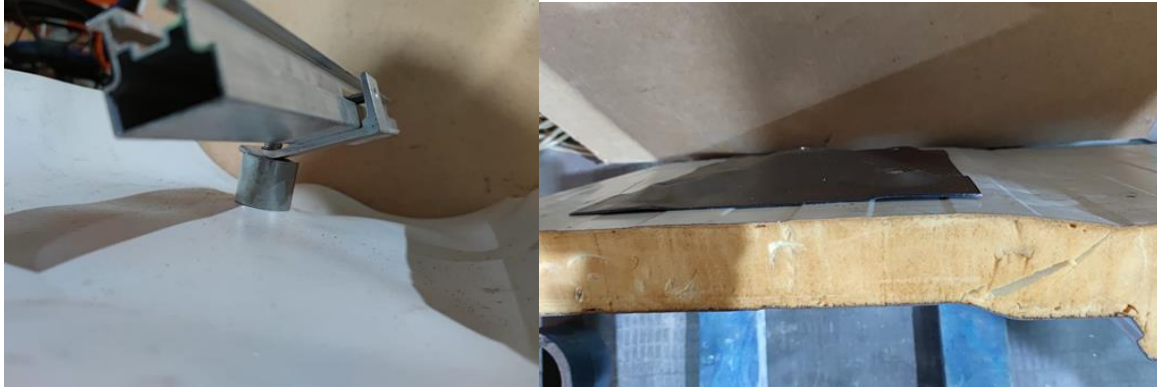
Figure 3b. Picture of NovaFlat specimen failure mode (System 2)
