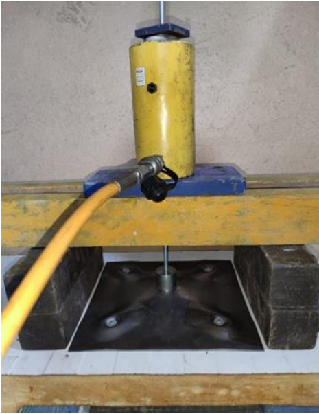
Figure 2a. Picture of NovaFlat specimen tensile test setup (System 1)
